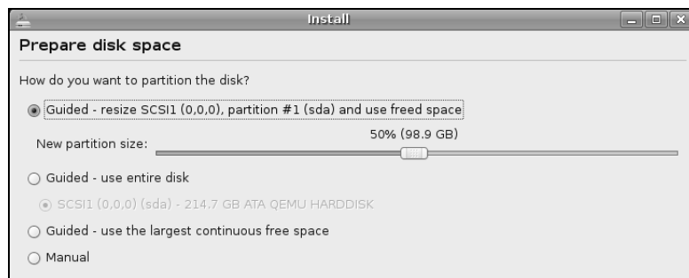
Figure 3-11 The Prepare disk space screen showing a hard disk with one partition and some free space
