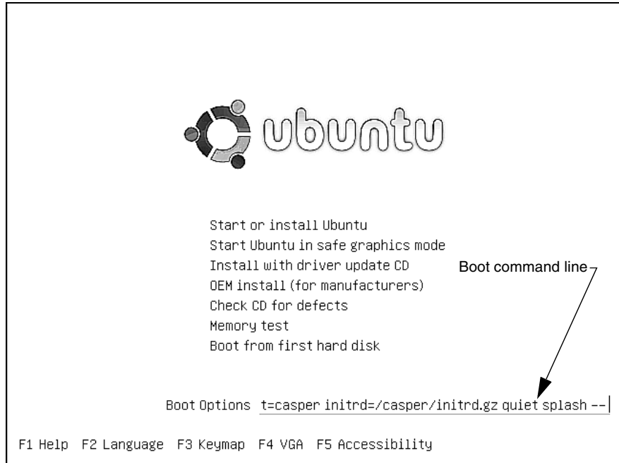
Figure 3-16 Initial install screen, F6 boot command line
